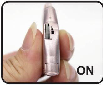
Insert a battery and completely close the battery compartment.
