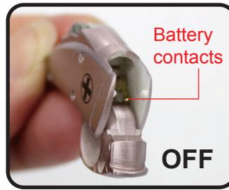
Open the battery compartment until the battery is no longer touching the battery contacts.
